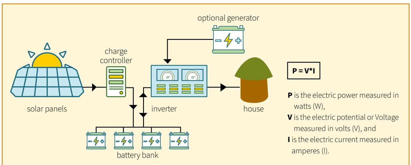
Figure 1: Elements of a typical SPS off-grid system
